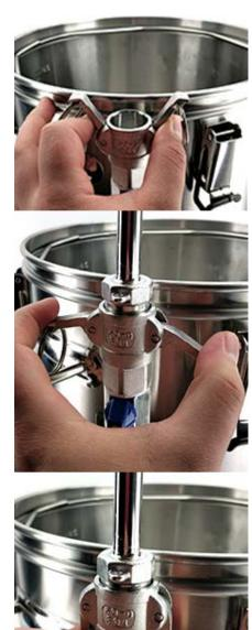
We must stress not to rotate the rotating racking arm while it is engaged in the lock down position. If you need to rotate the racking arm to fill your fermenter, please switch off the pump and readjust the camlock to the position you need then reengage the camlock.
