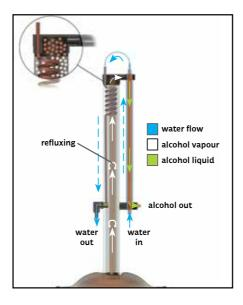
The saddles in the column provide a large surface area to maximise the contact between the liquid and vapour flows in the column, and accelerate the refluxing action.
