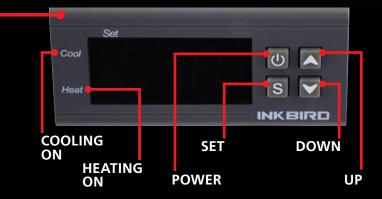
To change the settings hold the S button down till tS is showing (about 5 seconds). Using the up and down arrows find the setting you wish to check or change and press S. Set the new value with the up and down buttons and press S when finished. When all settings are correct press the power button to return to normal operation.
