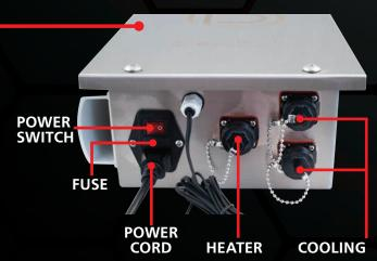
The power connectors are sealed with a water-tight cap. It is best to leave the caps in place when not in use. The connectors are polarity sensitive and will only go in one way. Once aligned correctly they push in and rotate clockwise 1/4 turn to lock.
