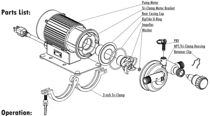
Connect the pump to your system using heavy wall and/or braided hoses. It is highly recommended to use  $\frac{1}{2}$ " ID x .125" wall silicone tubing. This hose will handle the pressures and temperatures of the beer brewing processes. Secure all hoses with clamps. If using NPT pipe fittings, always wrap the threads in Teflon tape to prevent galling of the threads. Galled threads are not covered under warranty.
